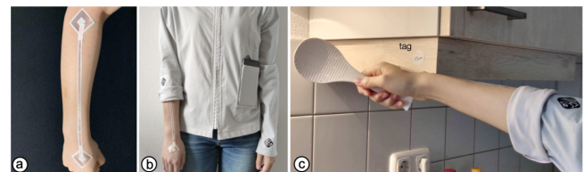
Figure 14: The elbow coil on the jacket is extended by an on-body relay sticker so the user can use her wrist to access a personal shortcut.
