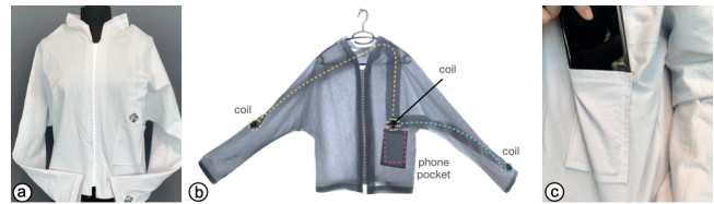
Figure 10: Proof-of-concept NFCe jacket: (a) results; (b) locations of the relays; (c) phone pocket.
